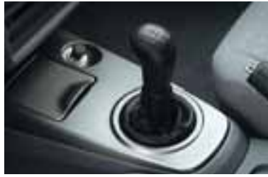
Leather-wrapped gearshift knob and parking brake lever (5MT) 20
