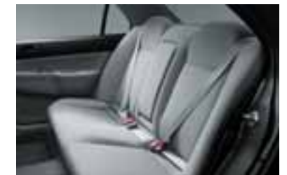
Rear 3-point ELR seatbelt and 2-point center lapbelt ☑06
