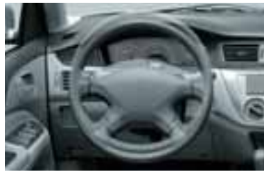
Tilt-adjustable steering column 21
