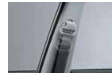
Height-adjustable front seatbelt anchors ☑05
